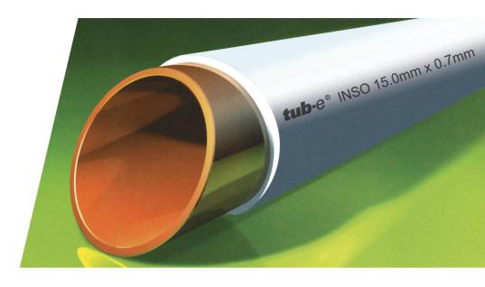
"**tub-**e° INSO" is a polyethylene coated copper tube, produced to comply to standard BS EN1057. The polyethylene coating is seamless, and it is most suitable **cold water services**. It also protects the tube during transport, installation and in the final application. The PE coating is manufactured in accordance with BS 3412, a specification for coverd copper tube.
