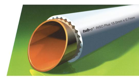
"**tub-***e*° INSO Plus" is a polyethylene coated copper tube, produced to comply to standard BS EN1057. The polyethylene coating is internally profiled with air channels to create a thermal barrier, and it is most suitable for **hot water service**. It reduces heat loss and minimizes the surface temperatures. It also protects the tube during transport, installation and in the final application. The PE coating is manufactured in accordance with BS 3412 a specification for coverd copper tube.
