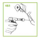
4. Push the pipe fully home into the fittings, slide the olive and nut up to the threaded part of the fitting and hand tighten the cap nut.
