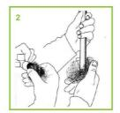
2 CLOSELY INSPECT ALL FITTINGS FOR ANY DEFECTS OR DAMAGE BEFORE INSTALLATION.
