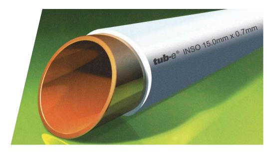
"  $tub-e^{\circ}$  INSO" is a polyethylene coated copper tube, produced to comply to standard BS EN1057. The polyethylene coating is seamless, and it is most suitable **cold water services**. It also protects the tube during transport, installation and in the final application. The PE coating is manufactured in accordance with BS 3412, a specification for coverd copper tube.
