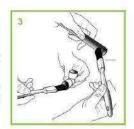
Apply a small amount of jointing compound around the pipe end and the outside of the olive or wind PTF tape three times around the thread of the fitting in an anti clockwise direction to ensure a water tight fit.
