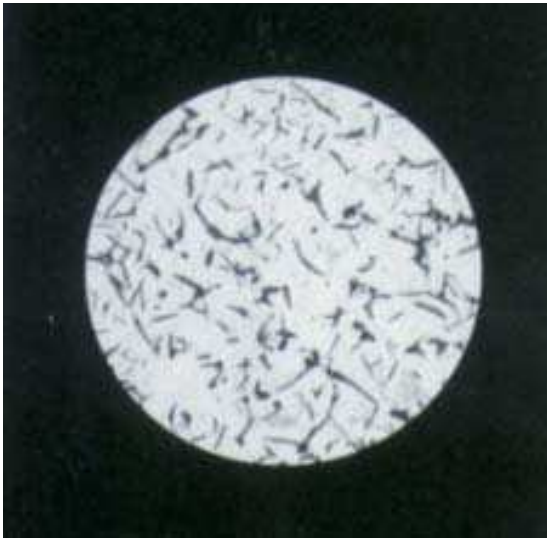
Microstructure of Cast Iron (Grey Iron)
