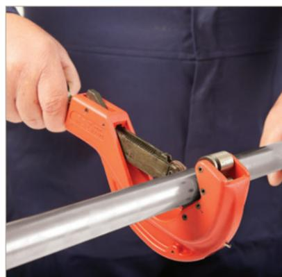
To cut the tube use a tube cutter, fine-tooth saw or a special electrical tube saw. It is important to ensure that the tube is cut completely square. Tube ends should be clean and free from scratches not less than the socket length.
