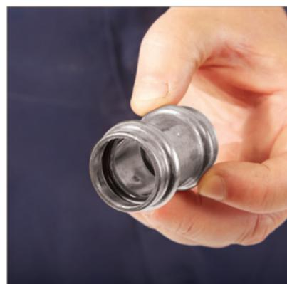
Inspect the fitting, checking the O-ring(s) are present and correctly seated and that the fitting is the correct size for the tube.
