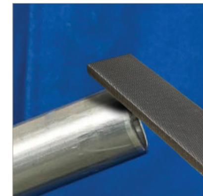
2. Make sure that the internal and external tube ends are free from burrs or sharp edges.
